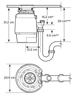
\*Distance from bottom of sink to centre line of disposer outlet. Add 12.7 mm when stainless steel sinks are used.
